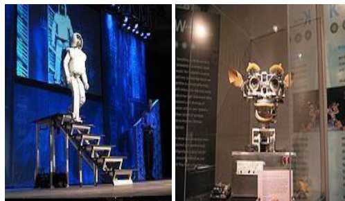
Fig 53.3 (a) ASIMO uses sensors and intelligent algorithms to avoid obstacles and navigate stairs. (b) KISMET , a robot with rudimentary social skills.
