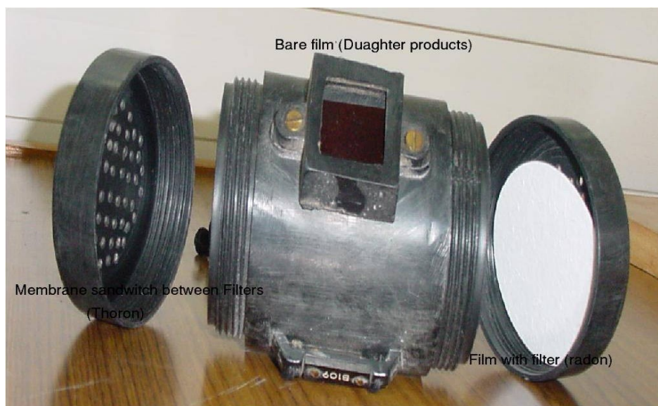
Figure.1 Schematic diagram and photograph of radon- thoron twin chamber dosimeter cup
