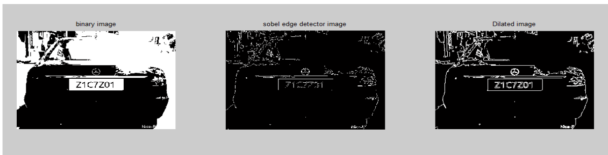
Fig.4 Sobel edge detection with dilation
